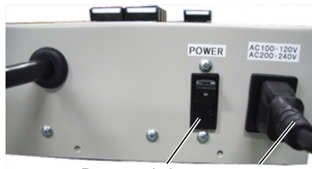
Power switch Power cable
